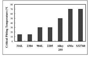
at a temperature appropriate for the alloy, shown in the graph above. If an artificial crevice is added to the sample the test measures crevice corrosion resistance rather than pitting resistance. The temperature which is just high enough to cause failure of this test is termed the Critical Pitting Temperature (CPT) or the Critical Crevice Temperature (CCT).
