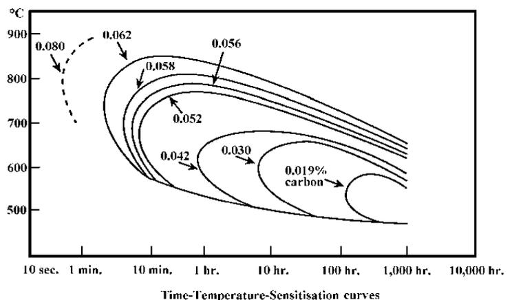
In the absence of sensitisation the corrosion resistances of the standard and “L” grades are usually identical.
