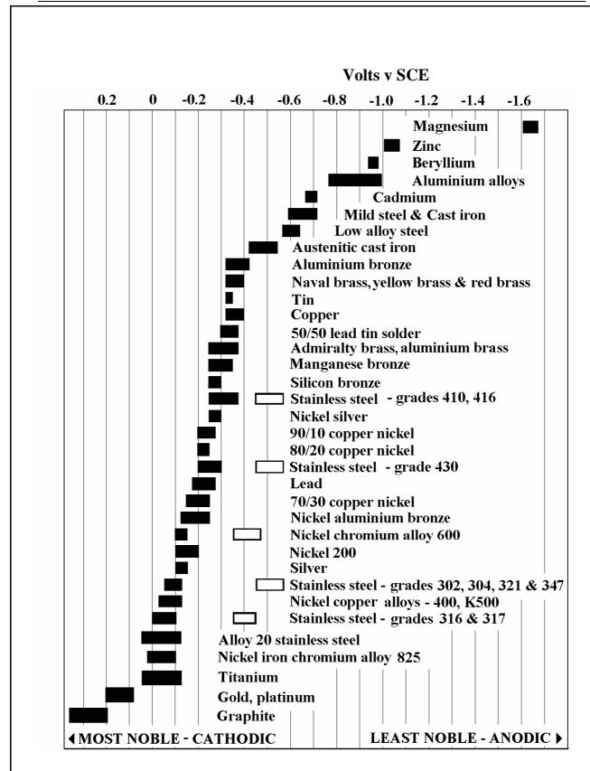
Corrosion potentials in flowing sea water at ambient temperature. The unshaded symbols show ranges exhibited by stainless steels in acidic water such as may exist in crevices or in stagnant or low velocity or poorly aerated water. The more Noble materials at the left side tend to be cathodic and hence protected; those at the right are less Noble and tend to be anodic and hence corroded in a galvanic couple.
