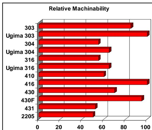
In general terms the three most important contributors to machinability of stainless steels are – **Sulphur content** – a steel with less than about 0.015% S will be more difficult to machine; almost all plate, sheet and pipe has this very low sulphur content. Round and hexagonal bar steels in common grades 304 and 316 are usually made with between 0.02 and 0.03% sulphur. Free machining stainless steels (eg grade 303) have about ten times this amount.
