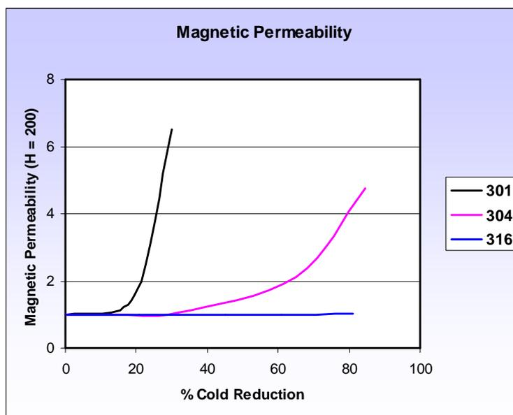
These comparisons are shown in the graph above. Note that different heats of steels of the same grade may exhibit different magnetic responses because of minor differences in the amounts of each element.
