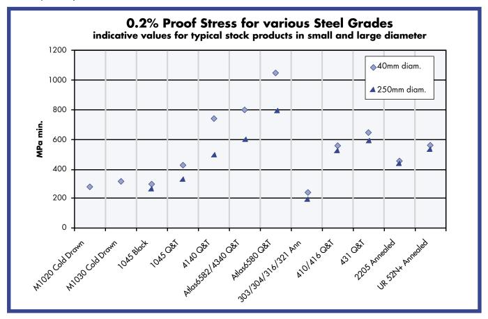
Atlas M1020 and M1030 have typical min. 0.2% proof stress values of 290MPa and 300MPa respectively in cold drawn condition for 40mm diameter bar. Cold drawn bar in these grades is available up to100mm. Cold drawn bar of 100mm diameter would generally have a 30MPa lower min. 0.2% proof stress than 40mm bar.
