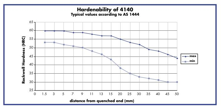
This test can also be used to specify hardenability of steel. Specifications for low alloy steels set down limits for hardenability by defining a maximum and minimum hardness at each distance from the quenched end, and the result is graphed as in the hardenability band for grade 4140. A Jominy test for a Heat of 4140 should give results between the two lines plotted on this graph.
