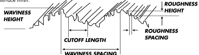
Deviation of surface shape from a straight line can be classified into two groups:
