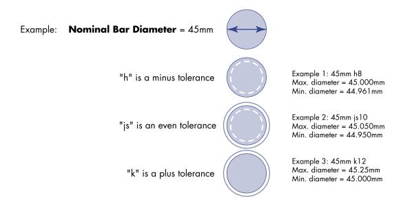
Note: k tolerances are according to the above table between k8 and k13 only.
