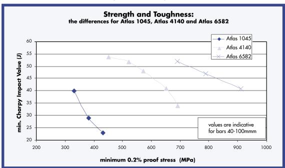
properties of this grade greatly deteriorate when hardened to higher strength. At comparable strength levels the minimum toughness of Atlas 4140 is about three times higher than that of Atlas 1045. This means that Atlas 4140 can absorb three times the impact needed to fracture Atlas 1045.
