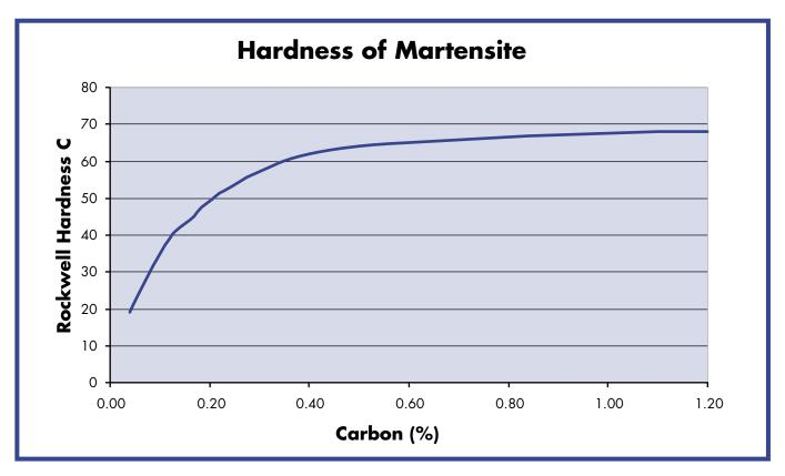
The cooling (also called "quenching") is carried out in various cooling media, with various cooling rates achievable. Quenching into brine (salty water) results in a very fast cool, plain fresh water gives a slightly slower cooling rate, and quenching into oil gives a slower rate again. Simply removing the hot steel from the furnace and cooling it by blowing air past it is slower still. A polymer quench is a synthetic water mix, with various cooling rates available.
