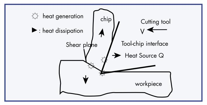
Optimising the metal removal rate therefore needs to be balanced against the negative aspects of excessive heat generation: shorter tool life and break-down of the tool. Generally, for carbon and alloy steels this is less of an issue than for stainless steels, which have a very low thermal conductivity and more heat tends to build up around the tool.
