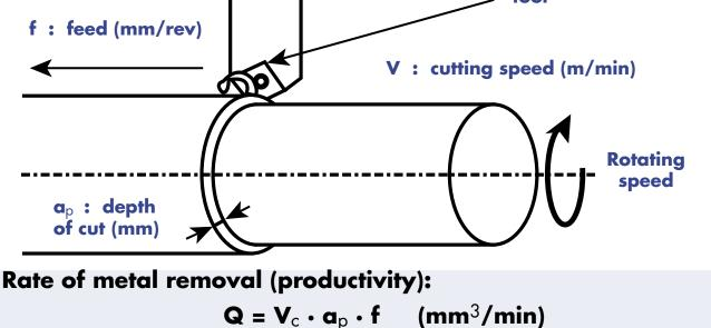
The rate of metal removal is one of the principal variables influencing overall productivity of the turning operation.
